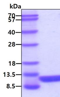
3 $\mu$ g by SDS-PAGE under reducing condition and visualized by coomassie blue stain
